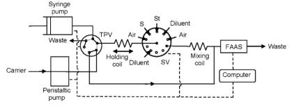
Fig. 1. Instrumental system developed for realization of CDM procedure in monosegmented sequential injection mode. St, standard; S, sample; TPV, two-positional valve; SV, selection valve.
