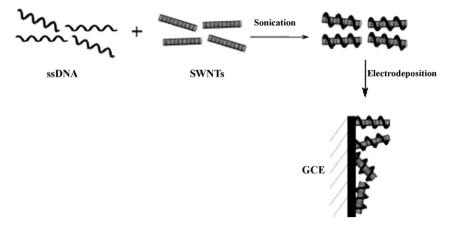
Scheme 1. The fabrication process of ssDNA–SWNTs modified GCE. First, ssDNA was mixed with SWNTs to form ssDNA–SWNTs hybrid, and then, the ssDNA–SWNTs hybrids were covalently deposited onto a glassy carbon electrode to form a uniform film.
