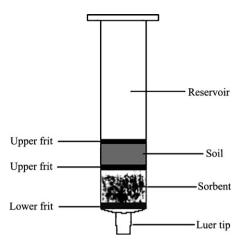
Fig. 1. SPE column packed with soil [24, modified].
