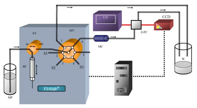
Fig. 1. Scheme of SIC set-up for determination of FC and PM. CCD: CCD UV-vis detector; MC: monolithic column; MP: mobile phase; MV: 6-port multi-position valve; PC: computer; SP: syringe pump; SV: solenoid valve; S1, S2, S3: Sample 1, 2, 3; UV: UV lamp, W: waste, Z-FC: Z-flow cell.
