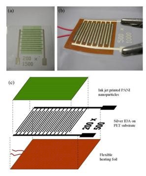
**Fig. 1.** Polyaniline interdigitated electrodes (nanoPANI-IDAs) shown alone (a) and with a thermofoil heater (b). Exploded schematic diagram of the nanoPANI-IDA electrode showing the different layers of the sensor (c).
