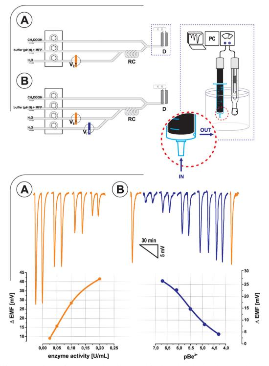
Fig. 2. FIA manifold for potentiometric detection of ALP activity (A) and ALP inhibitors (B) with fluoride ion selective electrode as detector. Typical FIAgrams and corresponding calibration graphs (insets) are given below.
