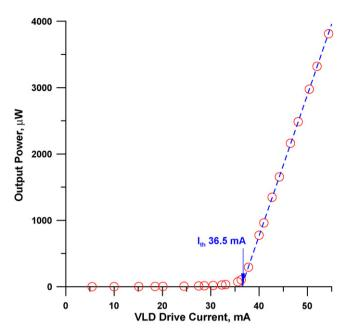
Fig. 2. Violet laser diode optical output vs. VLD drive current.
