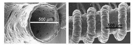
**Fig. 3.** Scanning electron microscopy (SEM) images of a ppy tube obtained by electrodeposition of ppy onto a 500  $\mu$ m diameter platinum wire, in a propylene solution containing pyrrole monomer, TBAPF<sub>6</sub> and 1% water, at -20 °C during 6 h.
