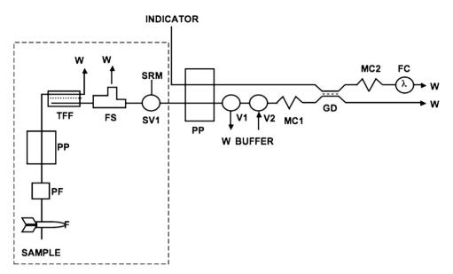
**Fig. 1.** Manifold diagram for total alkalinity analysis. Indicator (2.4 mL min<sup>-1</sup>); sample (2.4 mL min<sup>-1</sup>); PP, peristaltic pump; V1, valve 1 (miniature solenoid valve) feeds sample into the gas diffusion unit; V2, valve 2 pH 4.5 buffer reagent-injection; MC1 and MC2, 20 cm knotted mixing coils; GD, gas diffusion unit; FC, flow cell and flow through detector; W, waste.
