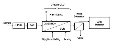
**Fig. 1.** Schematic flow diagram of HPLC coupled on-line with: diode array detector (DAD); chemifold for continuous flow (CF) system for on line oxidation of organic mercury to Hg<sup>2+</sup> and chemical vapor generator of Hg<sup>0</sup>; gas–liquid phase separator; atomic fluorescence detector equipped with miniaturized Ar/H<sub>2</sub> diffusion flame atomizer.
