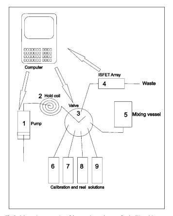
**Fig. 3.** Schematic presentation of the experimental system for the SIA multicomponent analysis. (1) Syringe pump, (2) hold coil, (3) multiposition valve, (4) sensor array with reference electrode, (5) mixing vessel, (6–9) individual solutions for mixing at different proportions.
