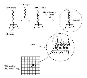
**Fig. 2.** DNA biochip with electrochemical detection. An unlabeled DNA-target chain hybridizes with a known electrode-bound DNA-probe chain. Further attachment of a hybridization redox label to the DNA duplex generates a current level that can be assigned to a known, specific DNA-probe sequence. The resulting current pattern in each spot corresponds to a certain level of gene expression.
