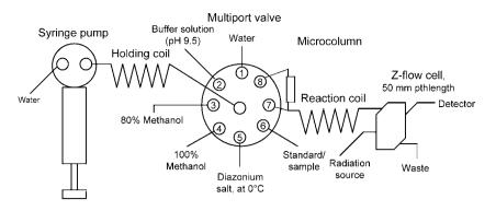
Fig. 1. Schematic diagram of a SIA manifold constructed for on-line solid-phase extraction, coupling reaction and spectrophotometric measurement for the assay of morphine in urine sample.
