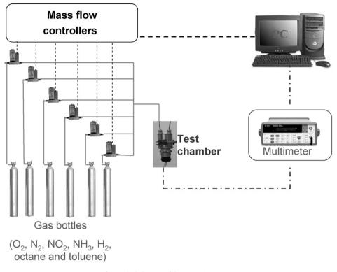
Fig. 2. Block diagram of the measuring system.
