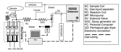
Fig. 1. MSFIA-CV-AFS system proposed for mercury determination.
