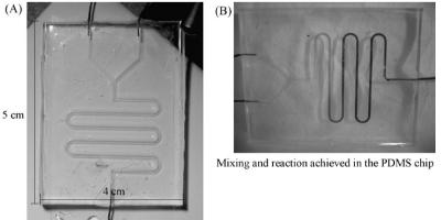
Channels: 700 µm wide by 700 µm deep
