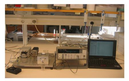
Fig. 1. Flow-through QCM system integrated with PC.
