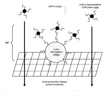
**Fig. 1.** Layout for DNA colorimetric detection with GNPs and latex microspheres. Free, red-colored ssDNA-functionalized GNPs freely move across the semi-permeable cellulose acetate membrane. White-colored latex microparticles, on the other hand, are too large to pass through that barrier. In the presence of an ssDNA-target, GNPs bind latex particles, generating large-size, red-colored conjugates, which become retained by the membrane.
