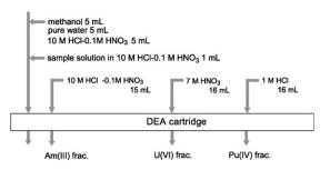
Fig. 1. Procedure for mutual separation of U(VI), Pu(IV), and Am(III) using DEA cartridge.
