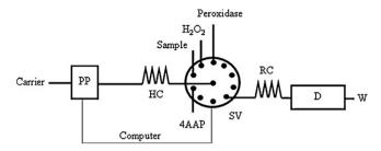
**Fig. 1.** SIA system. PP, peristaltic pump; SV, selection valve; HC, holding coil (4 m); RC, reaction coil (1 m); D, spectrophotometric detector; W, waste.
