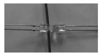
Fig. 4. Photograph of the LED detector used in this project.
