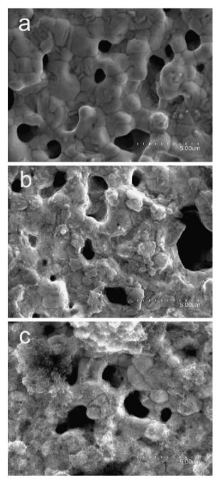
**Fig. 3.** SEM micrographs of (a) a sensor bare Au electrode, and of airbrushed (b) DWNT-COOH and (c) MWNT networks.
