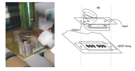
Fig. 2. A flow cell with reference electrode.
