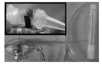
**Fig. 2.** Image of the first miniaturised pump developed in this work. The pump was constructed using Nafion-ppy actuators and the pump chamber was constructed using a 100  $\mu$ m thick PDMS film. The inlet and outlet were conical polyethylene peaces.
