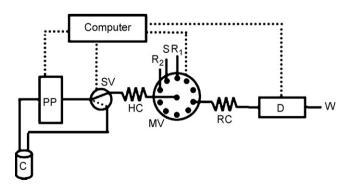
**Fig. 2.** SIA manifold for the determination of phenothiazines in aqueous and micellar media. C, carrier (H<sub>2</sub>O); PP, peristaltic pump; SV, solenoid valve; HC, holding coil (2 m/0.8 mm); R<sub>1</sub>, peroxidase 15  $\mu$ g mL<sup>-1</sup>; S, sample; R<sub>2</sub>, H<sub>2</sub>O<sub>2</sub> 5 × 10<sup>-4</sup> mol L<sup>-1</sup>; MV, multiposition selection valve; RC, reaction coil (1 m/0.8 mm); D, spectrophotometric detector (527 nm); W, waste.
