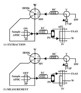
**Fig. 1.** SI-LLE system coupled to FAAS for lead determination. Two operation steps: (a) extraction (step 3) and (b) measurement (step 4). MV, multiposition valve; SP, syringe pump; V, syringe pump valve; PP, peristaltic pump; IV, injection valve; EC, extraction coil; HC, holding coil; PS; phase separator; DW, distilled water; W, waste.
