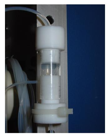
Fig. 2. Dual-conical micro-gravitational phase separator (PS).
