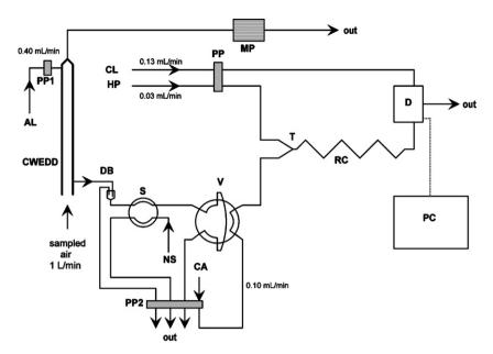
Fig. 1. Scheme of measuring apparatus. CWEDD, cylindrical wet effluent diffusion denuder; PC, computer; DB, glass–Teflon debubbler; PP, PP<sub>1</sub>, PP<sub>2</sub>, peristaltic pumps; MP, membrane pump; S, four-way solenoid; V, six-way injection valve; D, detector; RC, reaction coil; T, tee-piece; CA, deionized water; AL, absorption liquid; HP, hydrogen peroxide reagent; CL, chemiluminescent reagent; NS, nitrite standard solution.
