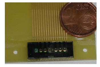
Fig. 1. A multisensor chip with sensitive membranes.
