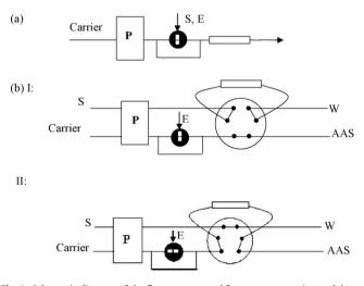
**Fig. 1.** Schematic diagram of the flow system used for preconcentration and determination of iron. (a) Single line FI system. (b) Two line FI system, I: sample loading; II: injection; S, sample; P, peristaltic pump; C, microcolumn and W, waste. Valve positions.
