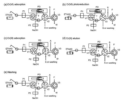
**Fig. 1.** Schematic illustration of the UV/nano-Au/TiO<sub>2</sub>-FI-ETAAS on-line system. ETAAS, electrothermal atomic absorption spectrometer; P1, peristaltic pump; V1, six-port valve; P2, microdialysis pump; T, micro-tee; PD, nano-Au/TiO<sub>2</sub> photocatalysis reduction device; V2, seven-port valve; S, sample; A, air; F, formic acid; V3, ten-port valve; W, waste. (a) Cr(VI) adsorption; (b) Cr(VI) photoreduction; (c) Cr(III) adsorption; (d) Cr(III) elution; (e) washing.
