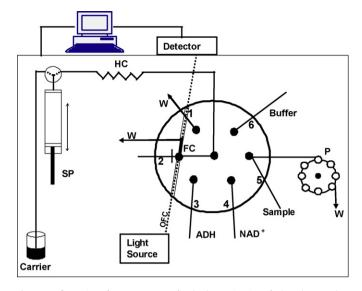
**Fig. 1.** Configuration of  $\mu$ SI-LOV system for the determination of ethanol; ADH, alcohol dehydrogenase 24 U mL<sup>-1</sup>; NAD<sup>+</sup>, cofactor 20 mM; Buffer, phosphate buffer pH 9.5; W, waste; Carrier, water; SP, syringe pump (2.5 mL); HC, holding coil; FC, flow cell; OFC, optical fibre cable; P, peristaltic pump; Detector, diode-array spectrophotometer.
